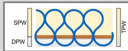
The surface pile weight is the technical relevant value according to EN 1307 and has to be mentioned in technical specification. As shown in the figure below alternatively to the total pile weight the surface pile weight can be used to calculate LCA results (IC<sub>x</sub>).
