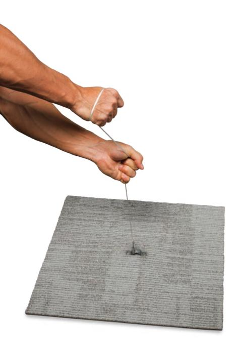
This string tile test demonstrates the dimensional stability of Interface's backing systems. The tile hugs the floor so that it's almost impossible to lift it while pulling straight up.
