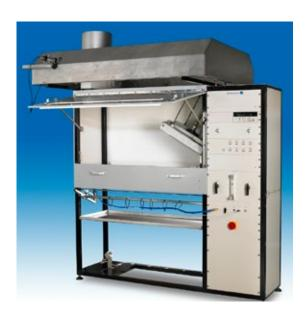
This European standard for the fire classification of construction products according to their reaction to fire tests lays down the classes for the flammability of floor coverings, which are now applicable throughout Europe. Further the CE Mark for floor coverings specifies the testing or classification of flammability according to EN 13501-1.
