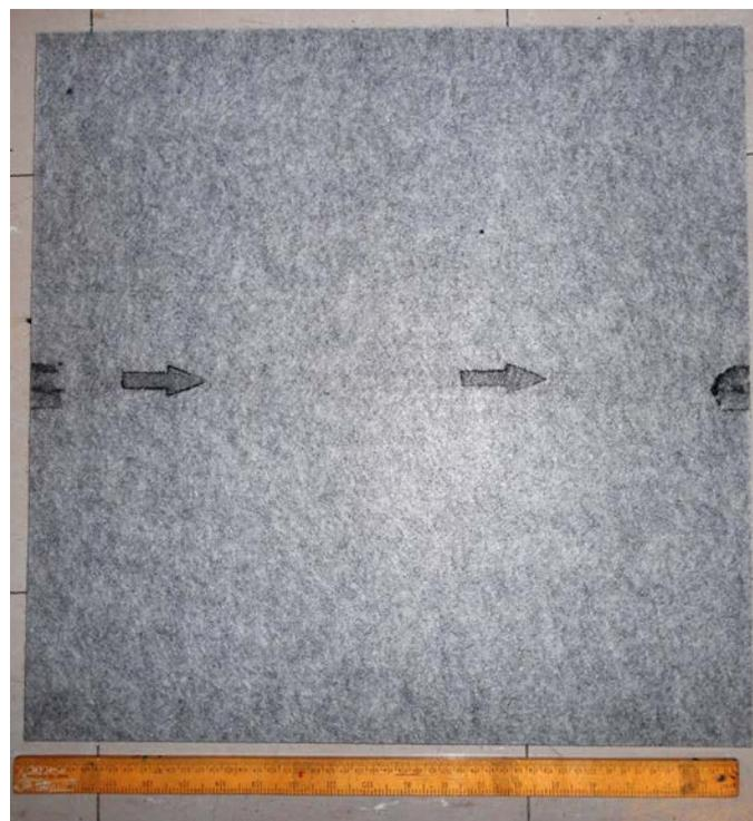
**Figure 2:** Interface PET CushionBacRE 780 g/m<sup>2</sup> 500mm x 500mm Carpet Tiles installed into the Reverberation Chamber for testing.
