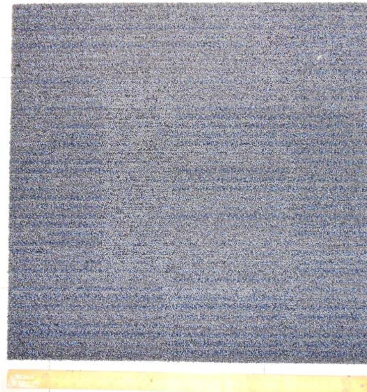
**Figure 2:** The underside of the Interface PET CushionBacRE 780 g/m<sup>2</sup> 500mm x 500mm Carpet Tiles
