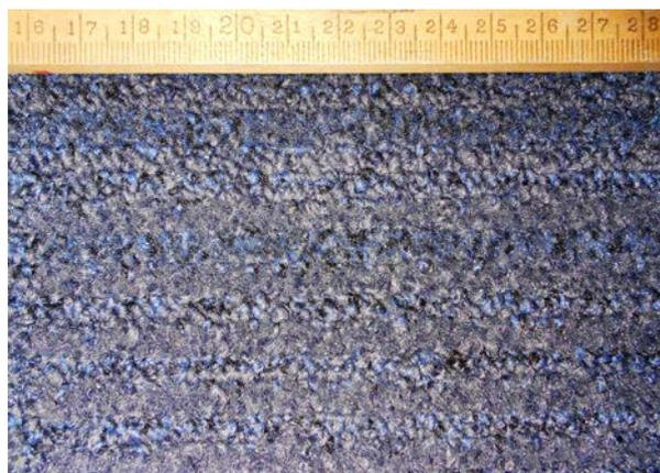
**Figure 1b:** The sound incident face of the Interface PET CushionBacRE 780 g/m<sup>2</sup> 500mm x 500mm Carpet Tiles.
