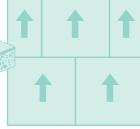
Offset the side joints of the tiles with arrows facing in the same direction.
