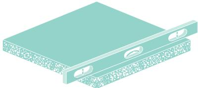
LES PLANCHERS BRUTS EN BÉTON NEUFS ET EXISTANTS DOIVENT ÊTRE CONFORMES AUX PLUS RÉCENTES VERSIONS DES NORMES ACI 302 ET ASTM F710 (PRATIQUE STANDARD POUR LA PRÉPARATION DU BÉTON RECEVANT UN REVÊTEMENT DE PLANCHER RÉSILIENT), PUBLIÉE PAR L'AMERICAN SOCIETY FOR TESTING AND MATERIALS : 171, RUE NEPEAN, BUREAU 400, OTTAWA (ONTARIO) K2P 0B4, 613 751-3409 / 100 BARR HARBOR DRIVE, PO BOX C700, WEST CONSHOHOCKEN, PA 19428-2959, ÉTATS-UNIS, 610 832-9585; [HTTP://WWW.ASTM.ORG](http://WWW.ASTM.ORG)
