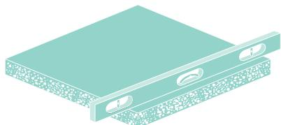
NEW AND EXISTING CONCRETE SUBFLOORS SHOULD MEET THE GUIDELINES OF THE LATEST EDITION OF ACI 302 AND ASTM F 710, "STANDARD PRACTICE FOR PREPARING CONCRETE FLOORS TO RECEIVE RESILIENT FLOORING" AVAILABLE FROM THE AMERICAN SOCIETY FOR TESTING AND MATERIALS, 171 NEPEAN RD, SUITE 400, OTTAWA, ON K2P 0B4, 613.751.3409 / 100 BARR HARBOR RIVE, WEST CONSHOHOCKEN, PA 19428; 610.832.9585; [HTTP://WWW.ASTM.ORG](http://WWW.ASTM.ORG)
