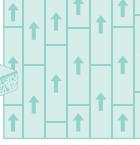
Offset the front and back tile joints. We recommend a variable drop ashlar for our Skinny Planks, as shown here, but our products can also be installed with a half drop ashlar.
