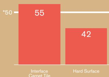
ASTM C423 **STANDARD TEST METHOD FOR SOUND ABSORPTION AND SOUND ABSORPTION COEFFICIENTS BY REVERBERATION ROOM METHOD**
