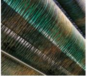
New post-consumer recycled content Type 6 or Type 6,6 Nylon fiber is returned to Interface and tufted into carpet face.
