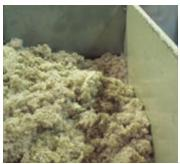
Separated Type 6 and Type 6,6 Nylon are sent to our fiber partners to be melted into its original chip form.
