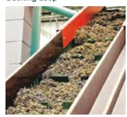
Reclaimed vinyl backing is shredded into small pieces and loaded into the agglomerator.
